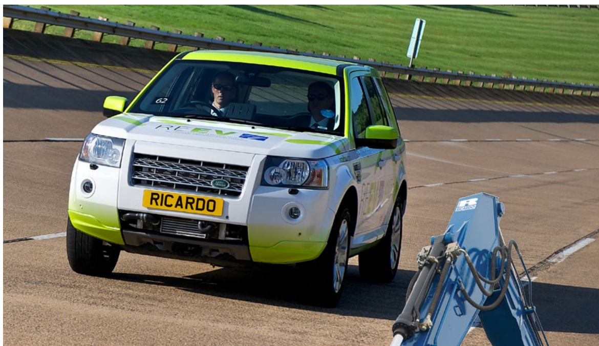
Range-extended electric vehicle based on a Land Rover Freelander uses downsized twin-cylinder engine and demonstrates potential for significant efficiency gains in the SUV sector
