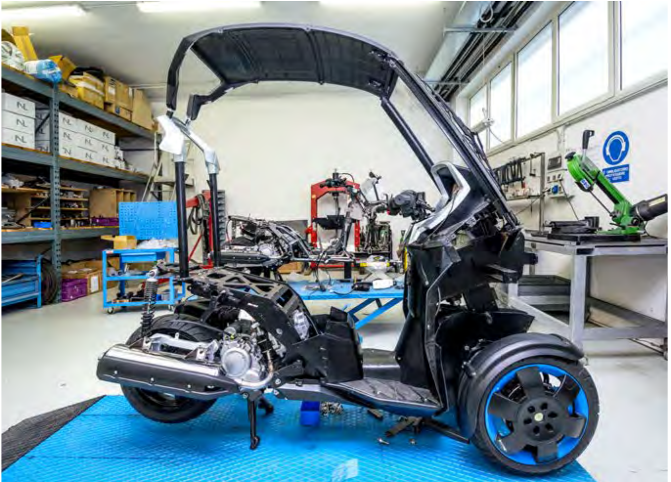
An advanced tilting design of a 3-wheeler personal transportation vehicle – incorporating a retractable roof – under assembly by Ricardo for ADIVA
