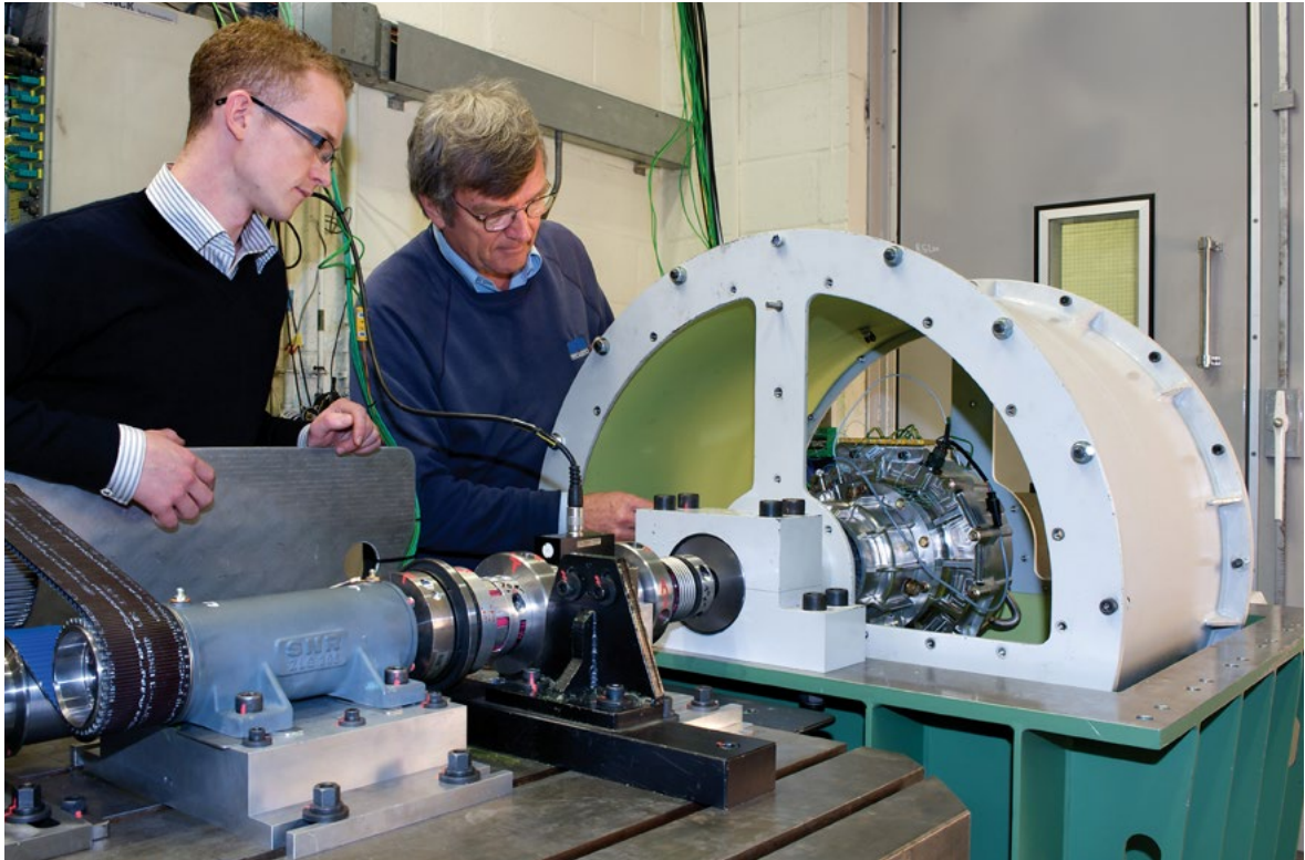
Testing of an earlier version of Ricardo's flywheel technology
