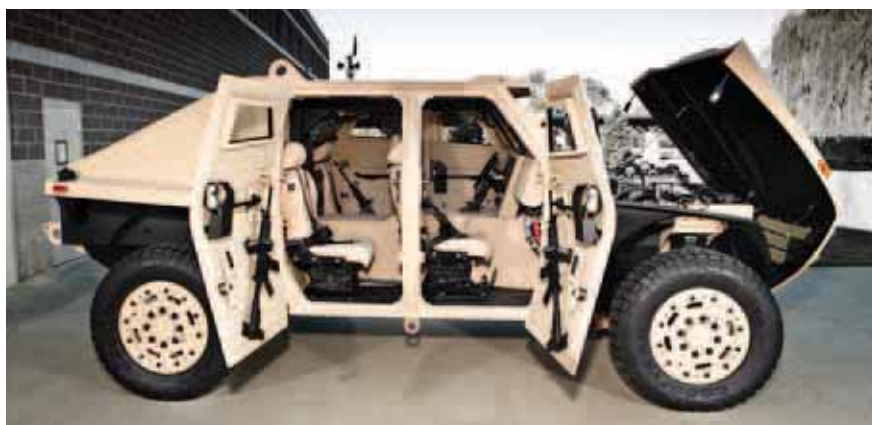
The body structure of the FED ALPHA makes extensive use of aluminium, reflecting the requirement for both strength and extreme fuel efficiency
